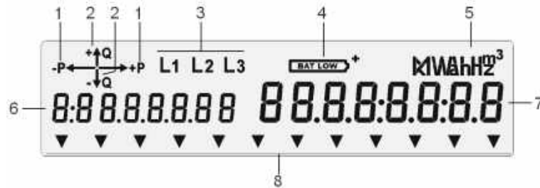
Figure 68 Basic layout of the liquid crystal display (LCD)
