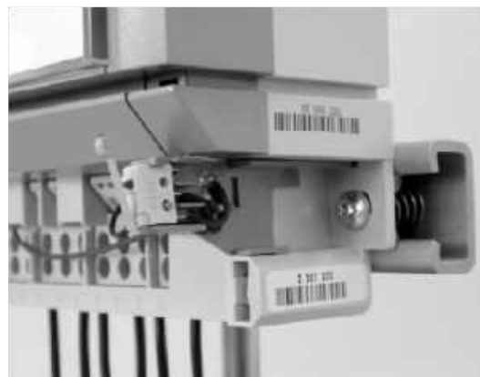
Figure 62 Fixing of cover detection unit to meter
