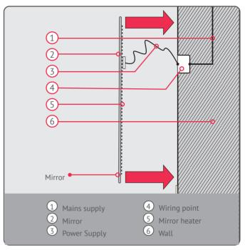
Step 4: Connect wiring and fix to the wall
