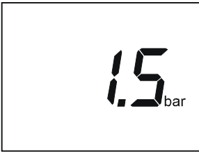
Fig.44 Boiler pressure value
